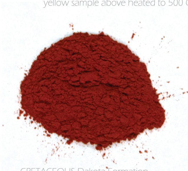
CRETACEOUS Dakota Formation Jefferson County, Nebraska yellow sample above heated to 500 C
